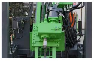
**NOTE:** When CSMF600 is used as diamond core drilling rig, the power head needs to be replaced with a 1600 Rotation head(As shown in the figure above).
