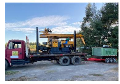
Water well drilling rigs are equipment used to drill water wells and are widely used in water resource development and water well construction. Its scope of use includes the following aspects:
