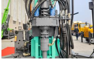
**NOTE:** When CSMF600 is used as Reverse circulation drilling rig and water well drilling rig, The power head is as shown in the figure.
